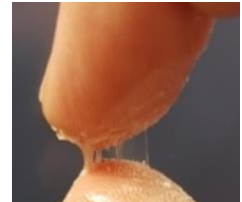
Illustration 2: Depending on temperature and humidity, the adhesive will soon start to develop a tack. Sometimes referred to as 'growing legs'
