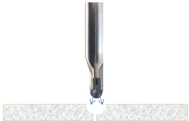
Hot air stream directed into the groove
