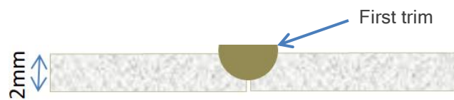
1 st pass with a Mozart knife with a spacer
