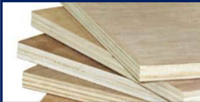
Plywood- thin ply's of timber glued together
