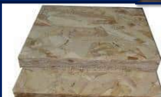
Strandboard- thin flakes of timber coated in resin that are glued and compressed
