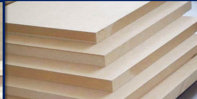
MDF- fine particles glued and compressed with wax and resins
