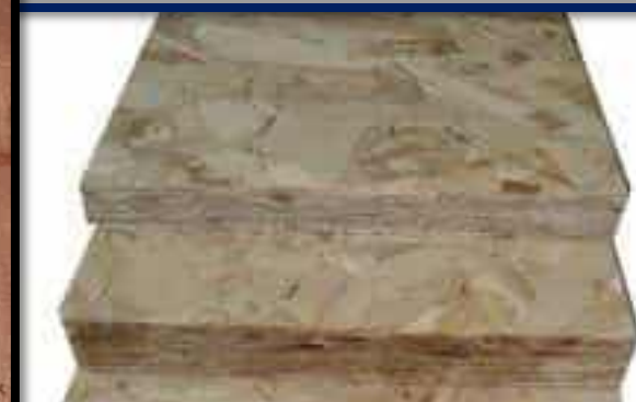
Strandboard - thin flakes of timber
