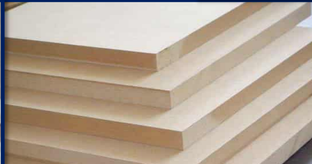
MDF- fine particles glued and
