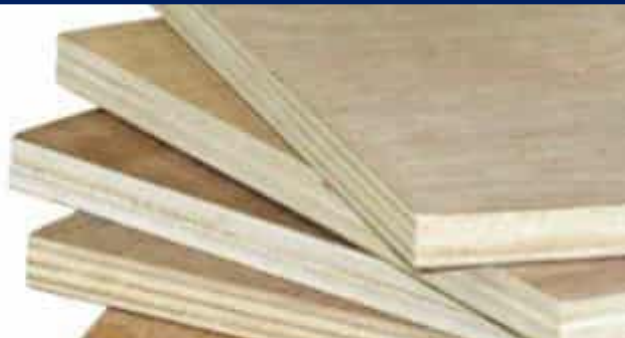
Plywood- thin ply's of timber glued together
