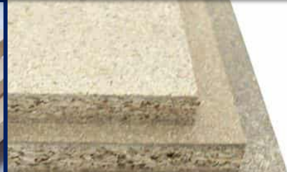
Particleboard - small chips of timber particles
