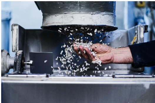
Recycled vinyl is chipped before being added back into the manufacturing process.
