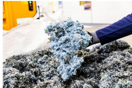
Fluff – high purity yarn (95%) – is generated by Tarkett's recycling center.
